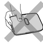
Do not cover the film ejection slot while printing.
